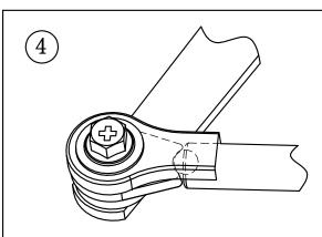
Opened the door to the desired hold -open position .Ensure the notch in cam and main arm seat' are properly engaged (to prevent slipping). Tighten the flange bolts by wrench .
