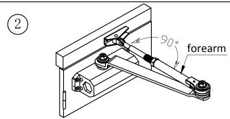
Adjust the length of forearm. To attach forearm to the door frame at 90° angle in accordance with the installation dimensions. Fix the foot in the corresponding position of door frame(the door should be closed), then tightened the locknut
